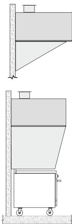
**Figure 12. Illustration of partial and full side panels.**
