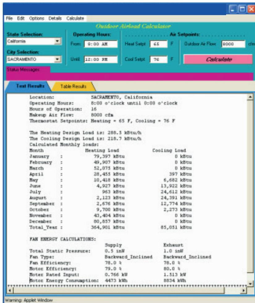
Figure 13. Sample output from Outdoor Airload Calculator screen.
